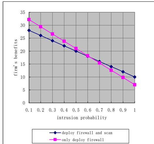
**Figure 3. Relationship between the firm's benefits and intrusion probability compared with (firewall, IDS) and firewall**
